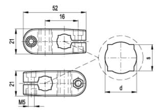
d = 14Rotation resistance = 5.5 s = 12Torque (N m) = 1100
